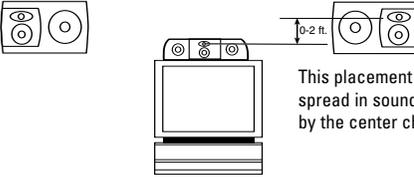
This placement provides a wide spread in sound, supplemented by the center channel speaker.
