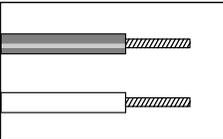
Speakers and electronics terminals have corresponding (+) and (-) terminals. It is important to connect both speakers identically: (+) on the speaker to (+) on the amplifier and (-) on the speaker to (-) on the amplifier. Wiring "out of phase" results in thin sound, weak bass and a poor stereo image. With the advent of multichannel surround
